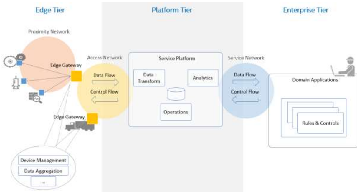
Figure 7-2 Three-tier IIS Architecture
