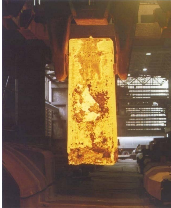
Annealed (1.250°C) steel slab, app. 150 t, process control and monitoring system made by FhG-IITB
